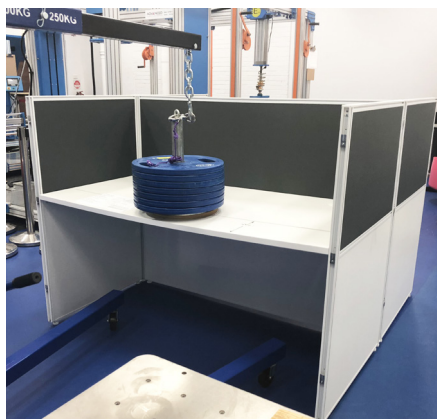
► Concentrated Static Load Test
